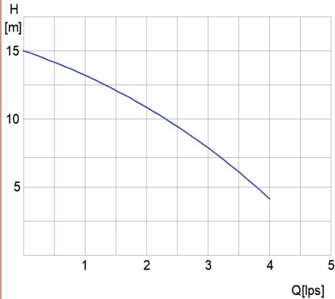
Performance Subjected to ISO 9906 GR3B-2012 Performance Curve
